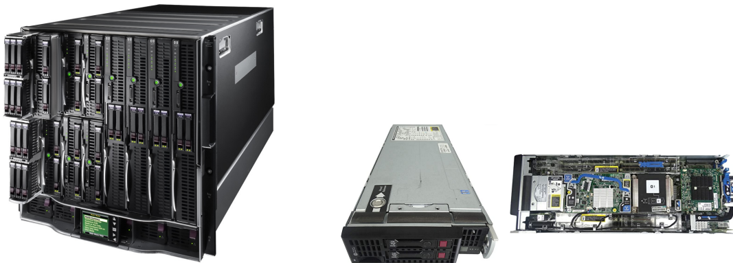
Figure 4.2: HP Blade chassi c7000 10U and one of the blade servers 2
