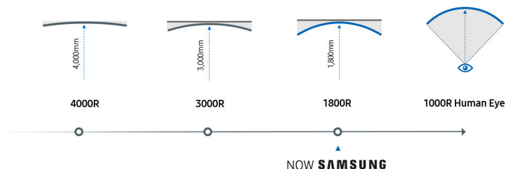
Figure 8.7: Curved screen, degree of curvature 6
