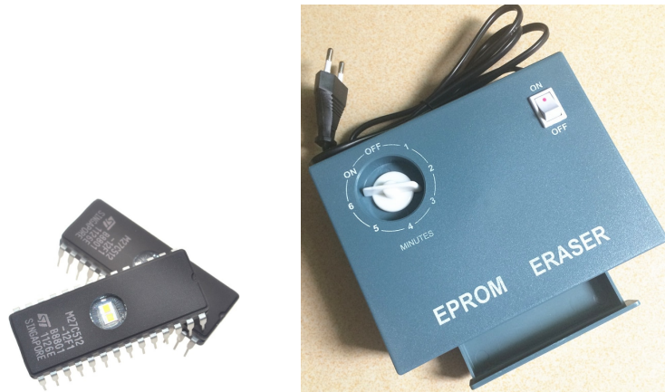
Figure 6.6: EPROM chip and EPROM eraser 3
