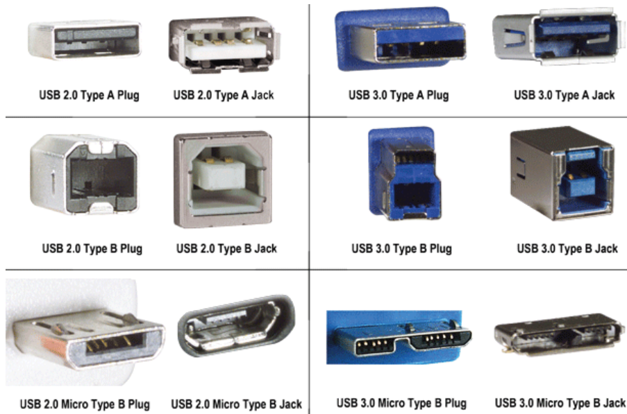
Figure 3.1: USB type A and B connectors and plugs 1
