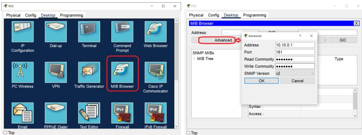
Request some of the device parameters (for simple variables, use the GET method, for table variables, use the GET BULK method):
